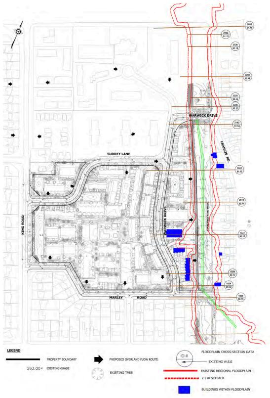
Figure 47 - Existing Floodplan Mapping
