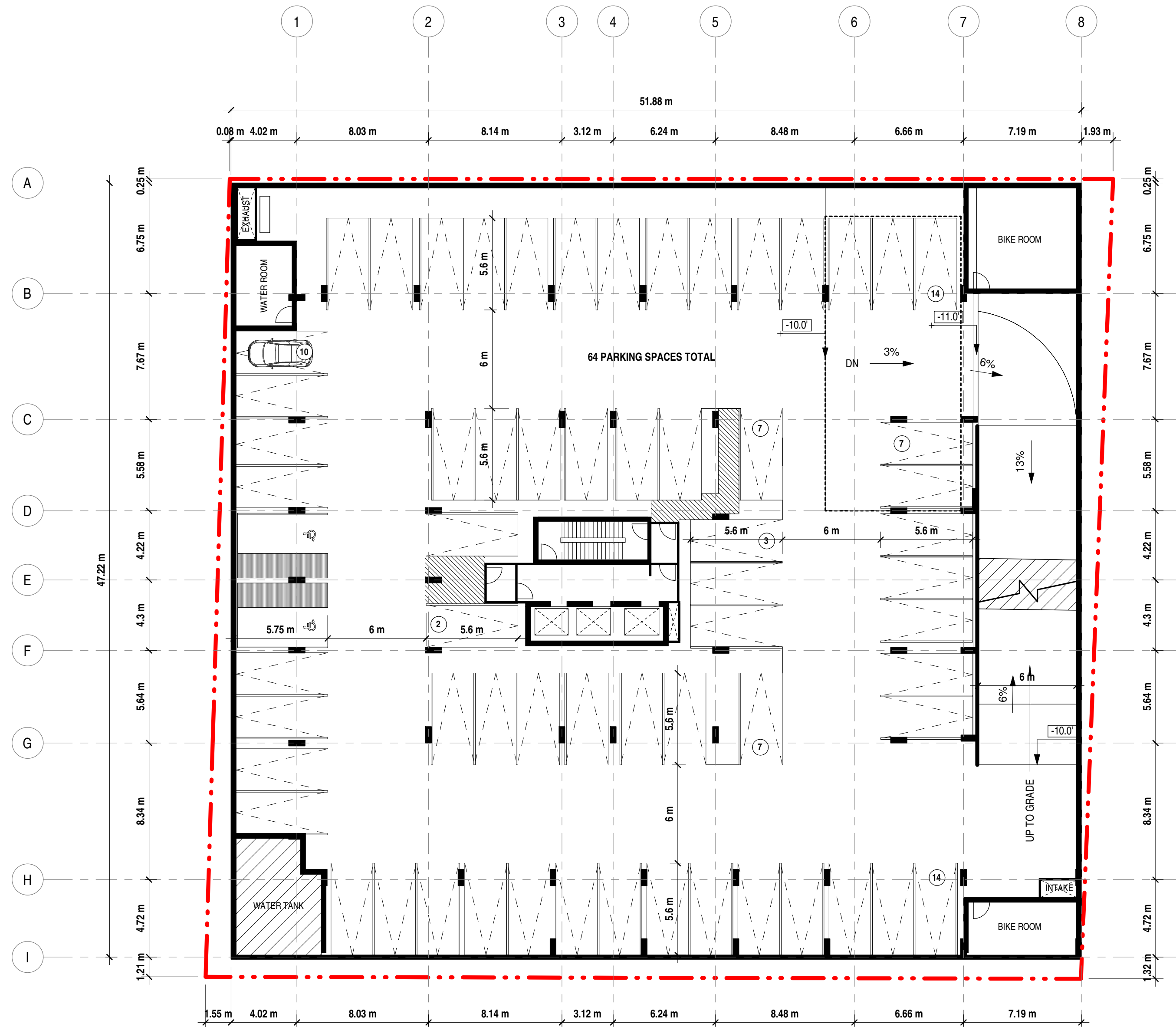
LEVEL B1 FLOOR PLATE: 25,330sf (2353sqm) 64 PARKING
