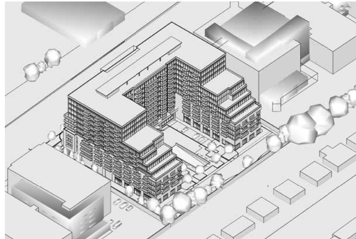
Figure 11: Axonometric View Looking Northeast Showing Terracing Strategy - Generated from the 3D Model Prepared by Terry Martino Architects
