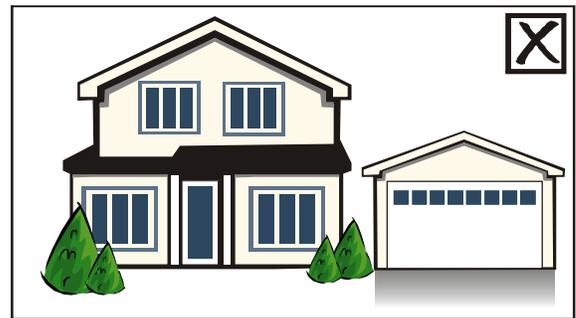
Fig. 4.2 - Garage elevation greater than 50% of dwelling facade
